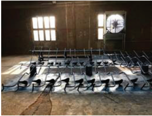
Components of overhead manned cableway devices
